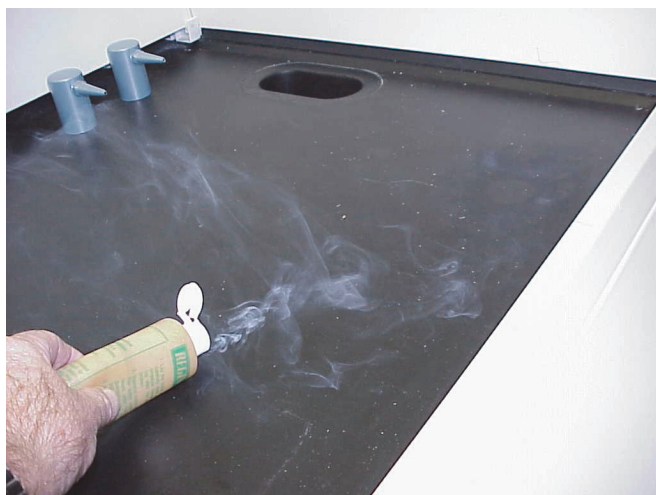
FIGURE 3.2 Lazy airflow as demonstrated by smoke visualization.
