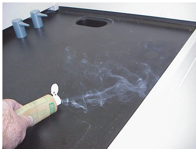
FIGURE 3.3 Reverse airflow as demonstrated by smoke visualization.
