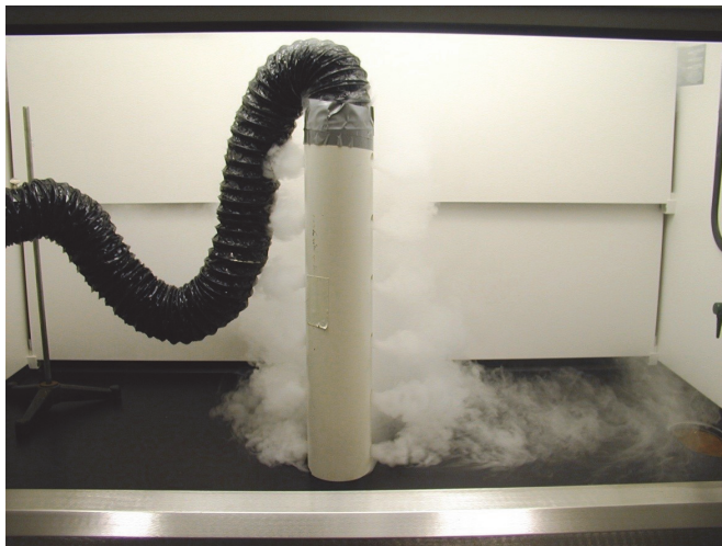
FIGURE A.2 Cylinder diffusion of smoke from smoke generator.
